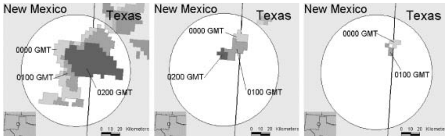
Figure 1. Boundary effects on object characterization. The three frames show rainfall areas defined using 0, 2, and 4 mm thresholds. Note the size, shape, and direction of movement varying by threshold.
