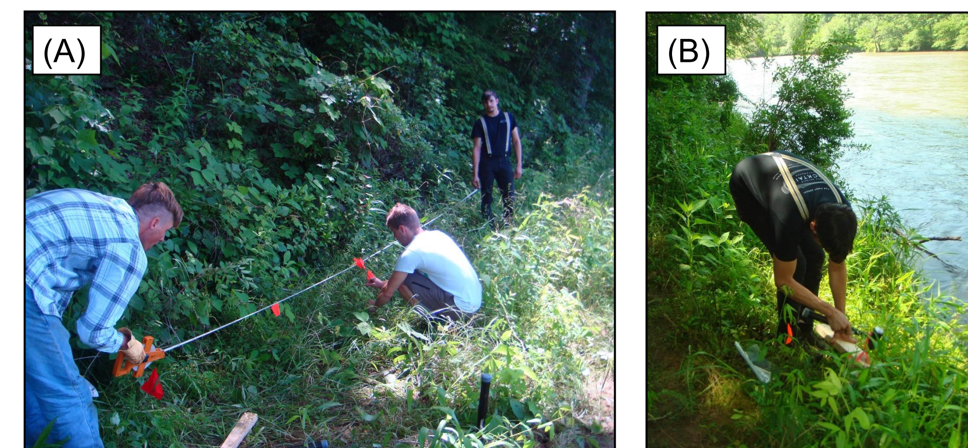
Figure 3: (A) Field crew measuring one meter increments to the right of the surveyors tape and (B) member of crew using a sledge hammer and 2 x 4 to drive PVC pipe into ground. Photos by Anna K. Boeck 2013.
