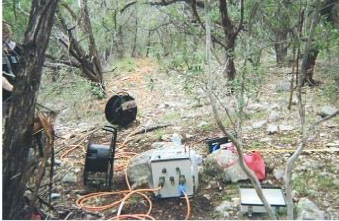
Figure 1a. The set up of the line once the conductive wires are set into place, in line with the electrodes. The meter and battery are located at the bottom center and right.
