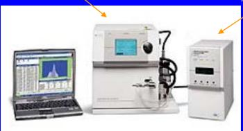
Condensation Particle Counter (CPC): Total Particle Number Concentration
