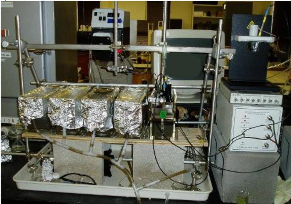
Aluminum support and micromanipulator used to hold electrodes in place
