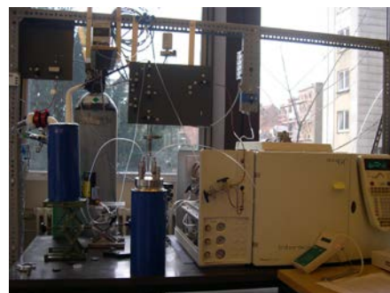
Figure 13 : The DMS/P analytical scheme applied for ice samples at the University of Brussels. A similar system has been used during SIMBA.
