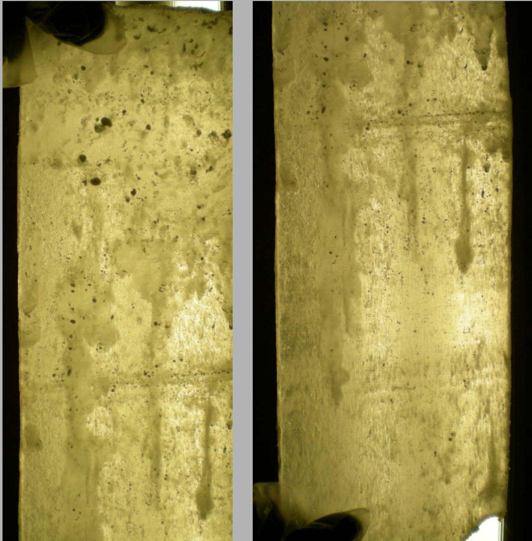
Figure 8 : 1 cm-thick section of the Brussels 4 core clearly showing the descending refrozen brine tubes. Fingers for scale.
