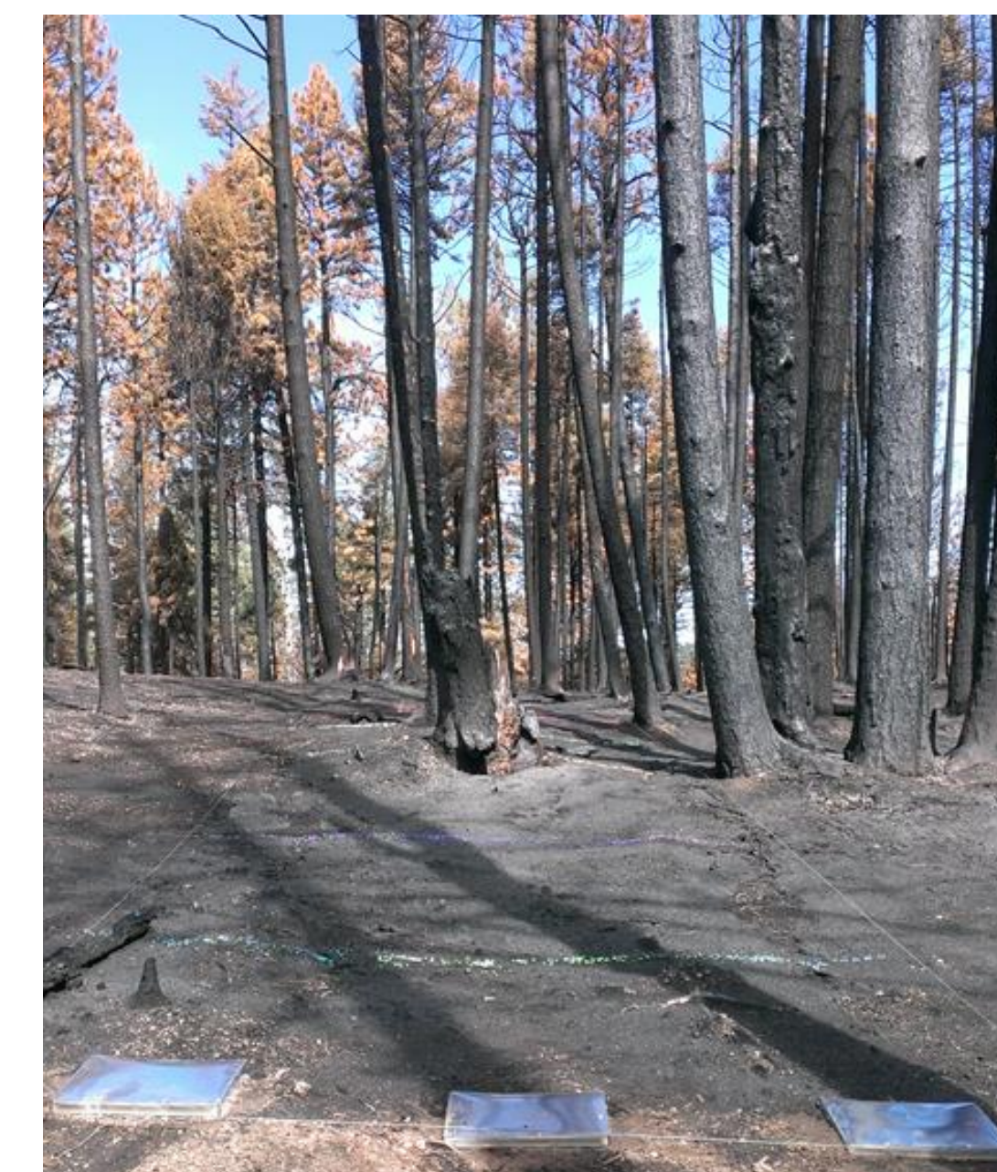
Fig 4. A high severity erosion plot after seed tracers had been dispersed. Three sediment traps measuring approximately 40 x 30 x 20 cm, were installed downslope of each erosion plot.
