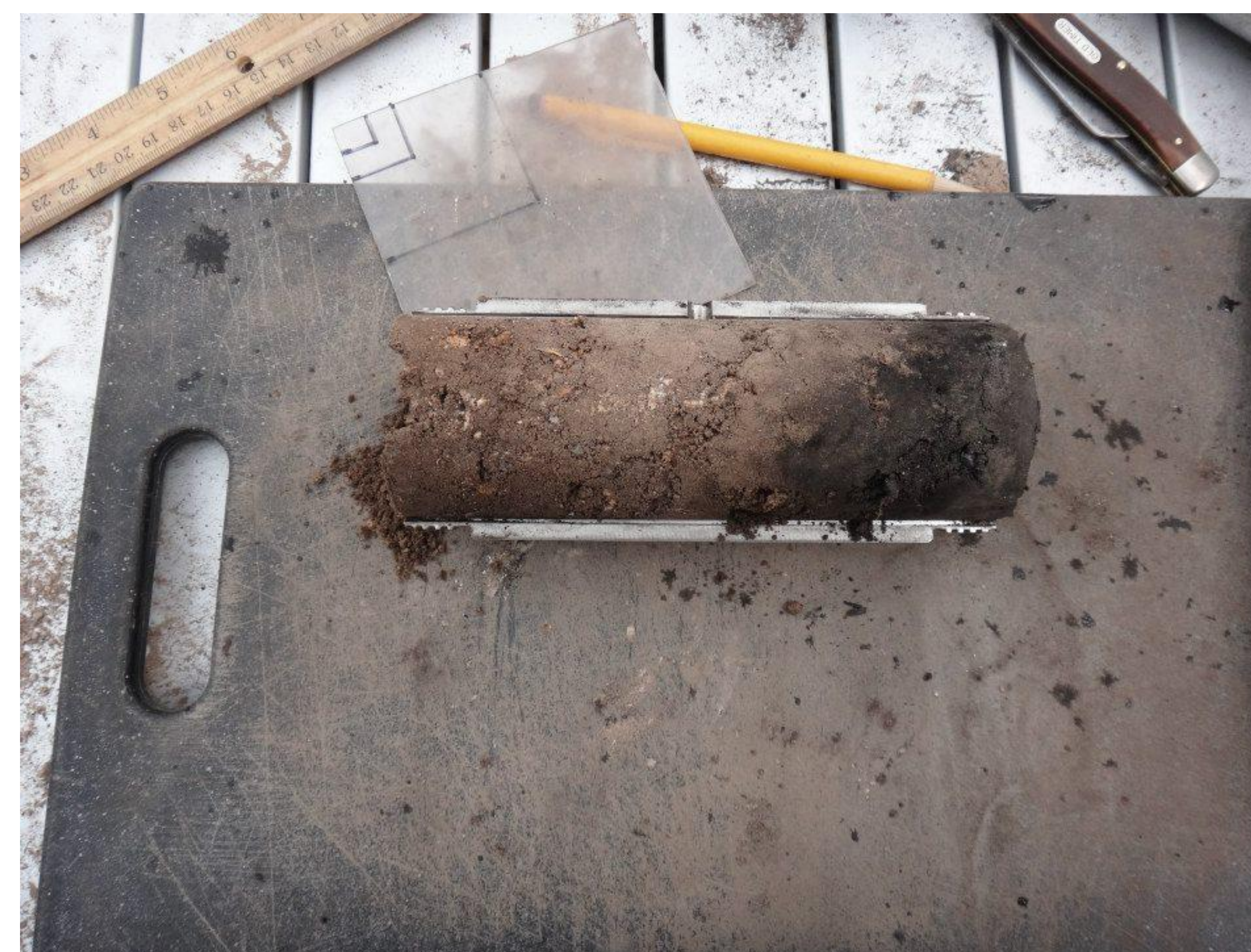
Figure 3. A soil core sub sample from a severely burnt site with the burnt soil surface on the right. The core is 15 cm long. The top 10 cm are divided into five 2 cm increments and the rest is discarded.
