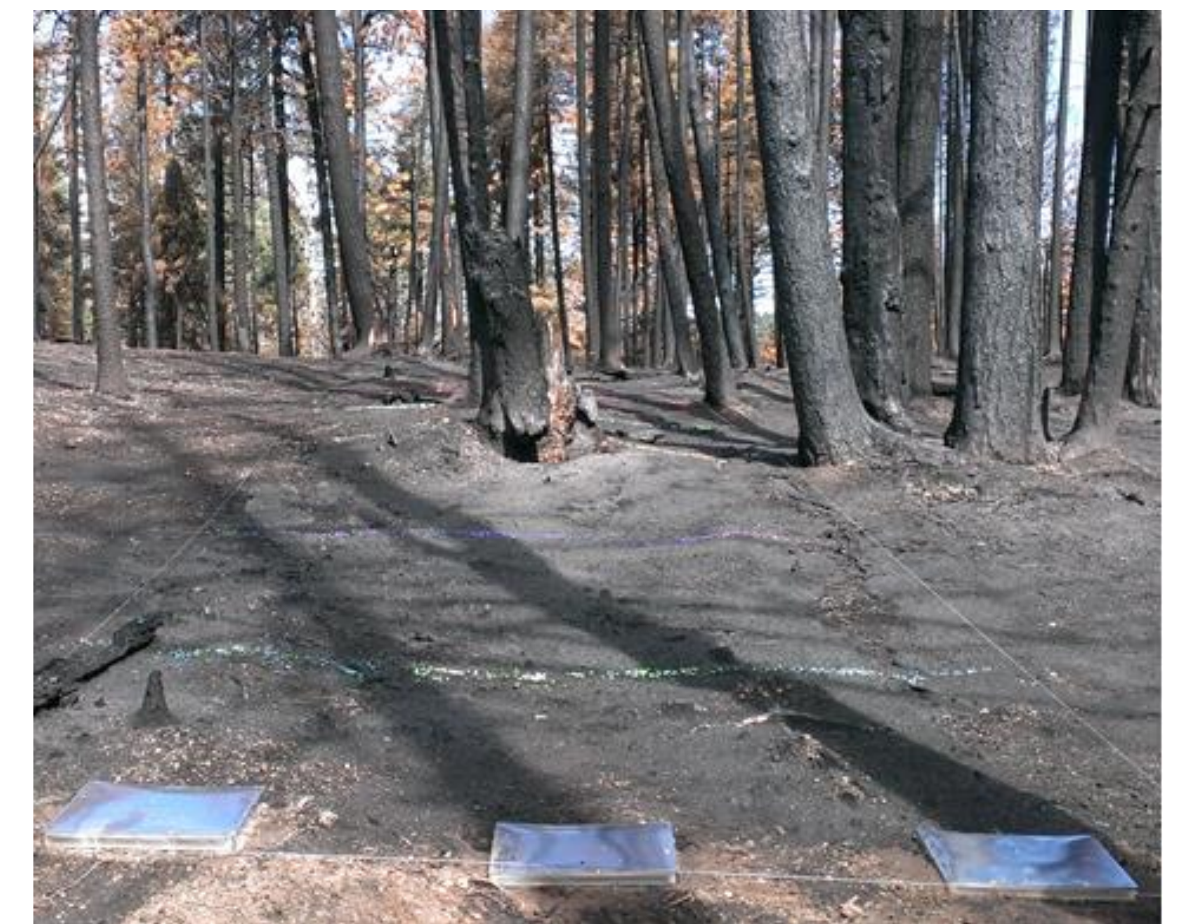
Figure 4. A high severity erosion plot with three sediment traps measuring approximately 40 x 30 x 20 cm, installed downslope of the plot.
