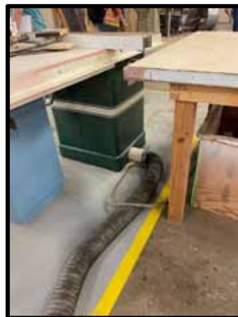
PHOTOGRAPH 186 - Dust collector connected to woodworking machine
