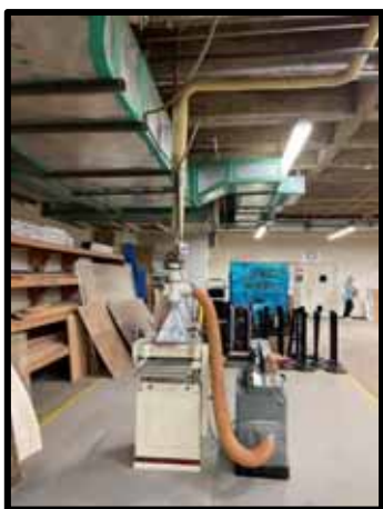
PHOTOGRAPH 187 – Dust collector drop connected to woodworking machine
