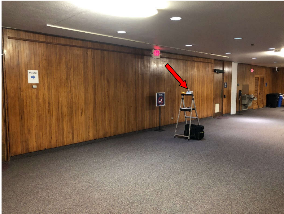
PHOTO 1: Shows airborne mold sample BZ-01, indicated by the red arrow, collected from the normal breathing zone in Corridor 1.01 by Restroom 1.01.04A.
