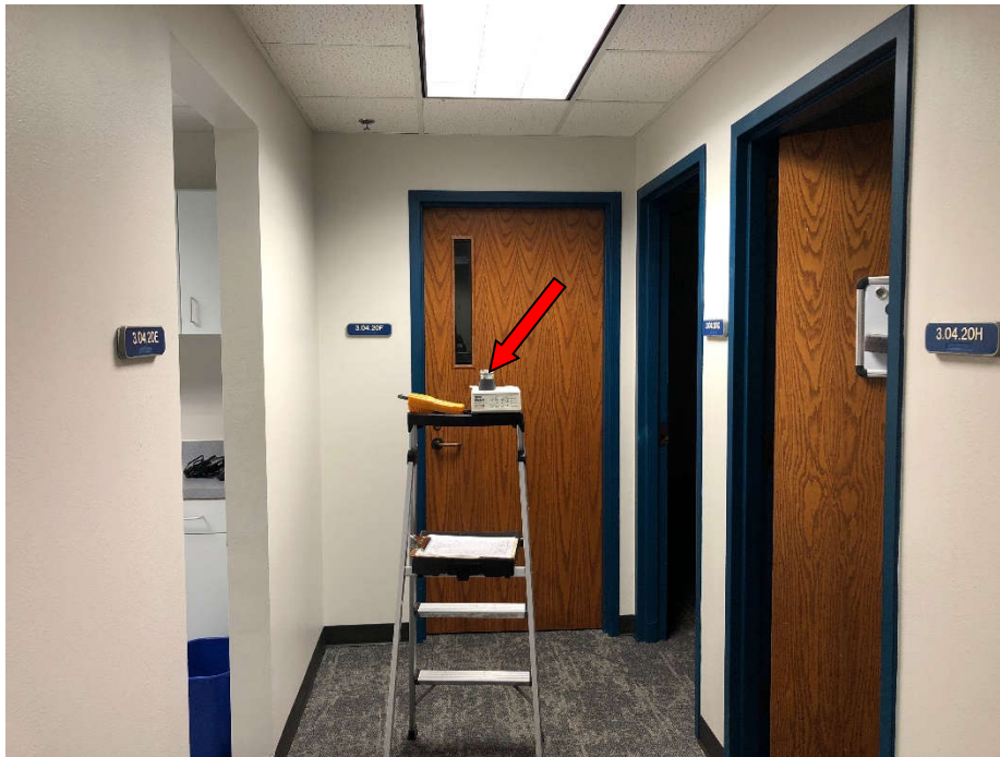
PHOTO 11: Shows airborne mold sample BZ-11, indicated by the red arrow, collected from the normal breathing zone in Room 3.04.20.
