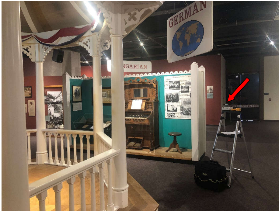
PHOTO 19: Shows airborne mold sample BZ-19, indicated by the red arrow, collected from the normal breathing zone in Corridor 2.05.
