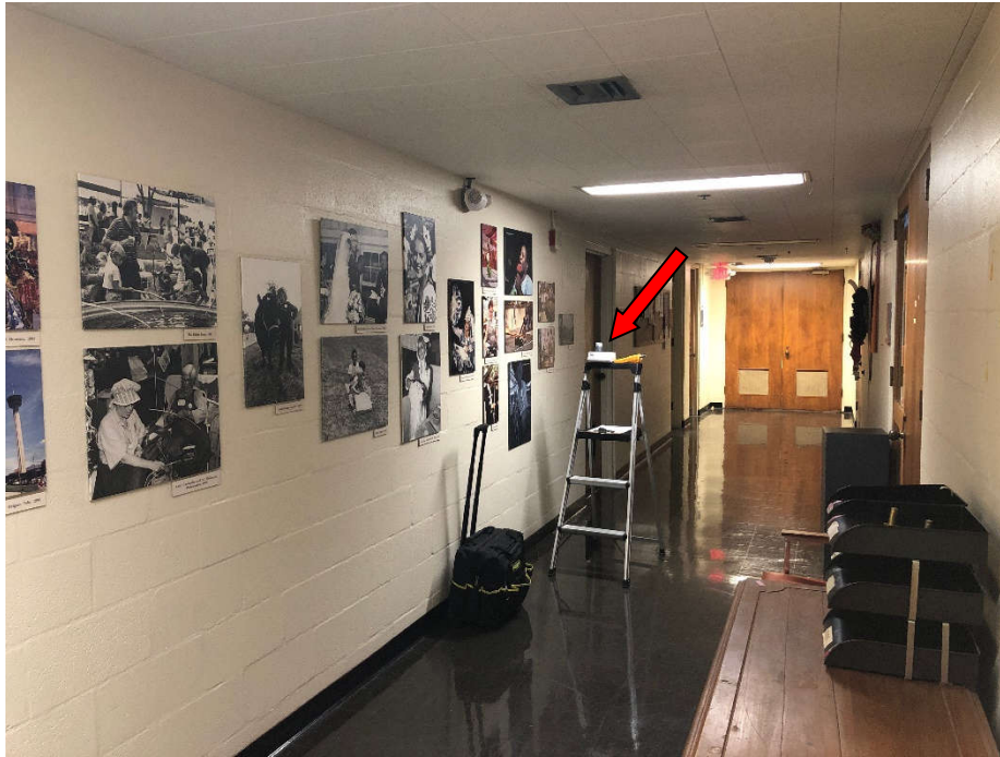
PHOTO 3: Shows airborne mold sample BZ-03, indicated by the red arrow, collected from the normal breathing zone in Corridor 1.03A by Room 1.03.03.
