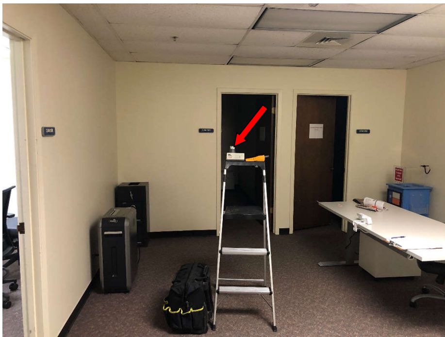
PHOTO 12: Shows airborne mold sample BZ-12, indicated by the red arrow, collected from the normal breathing zone in Room 3.04.10.
