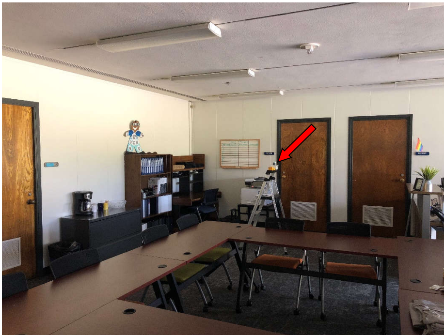
PHOTO 6: Shows airborne mold sample BZ-06, indicated by the red arrow, collected from the normal breathing zone in Room 1.01.03.
