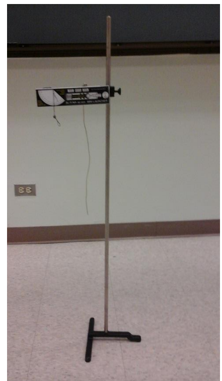
Illustration 1: When performing measurements such as range and launch height, always measure from the crosshatch, ie, the 'Ball Center of Mass' as shown in this picture.
