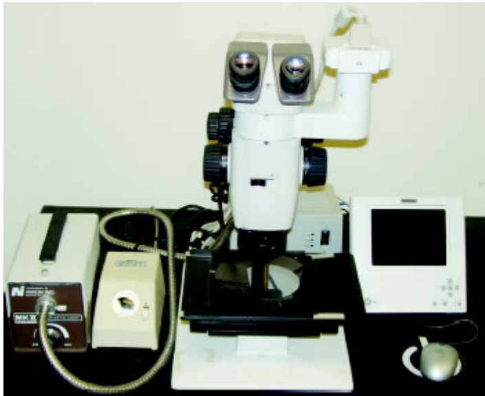
Figure 2. Nikon SMZ-U microscope
