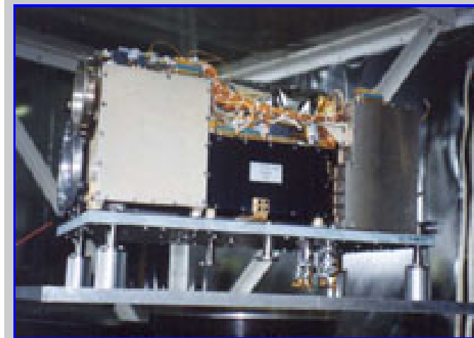
The optics and electronics of the OMEGA instrument
